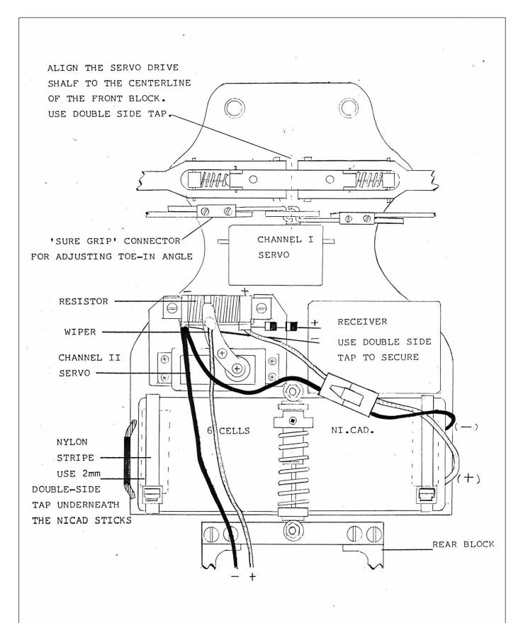
POSITIONING OF R/C SET AND NI-CAD. BATTERY
